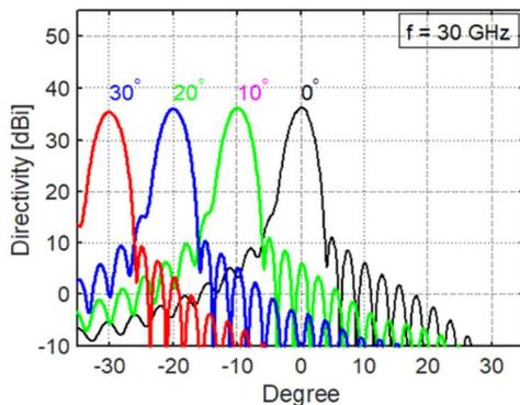
Figure 1 Torus reflector scan performance.
